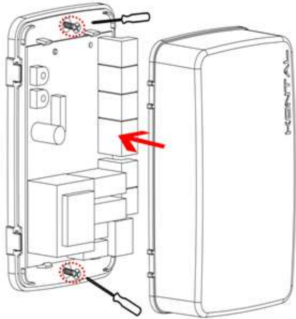
Figure 6.2 Screwing the GAF onto a flat surface
